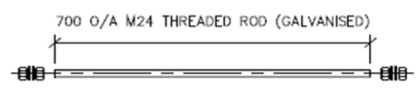
ENLARGED DETAIL OF M24 H.D. BOLT THREADED ROD TO BE SUPPLIED COMPLETE WITH 4-NUTS AND 4-WASHERS (SCALE 1:10)
